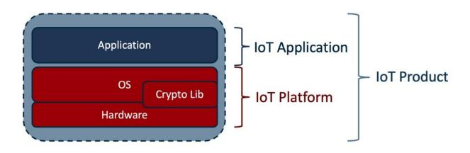
An **IoT Platform** is the hardware/software providing an operating environment for an IoT Application. IoT Platforms parts can be developed and evaluated separately, for example by evaluating the cryptographic library, an OS, hardware, and then combining them. In terms of the Common Criteria, the IoT Platform (part) identified in the ST is our TOE.
